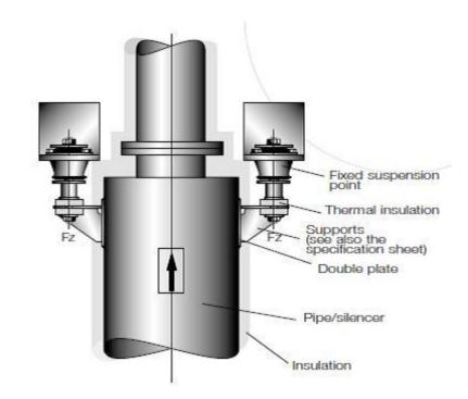
Mounting principle: horizontal set-up
